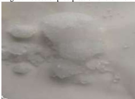
Fig. 2: Alum crystal formed after washing and drying
